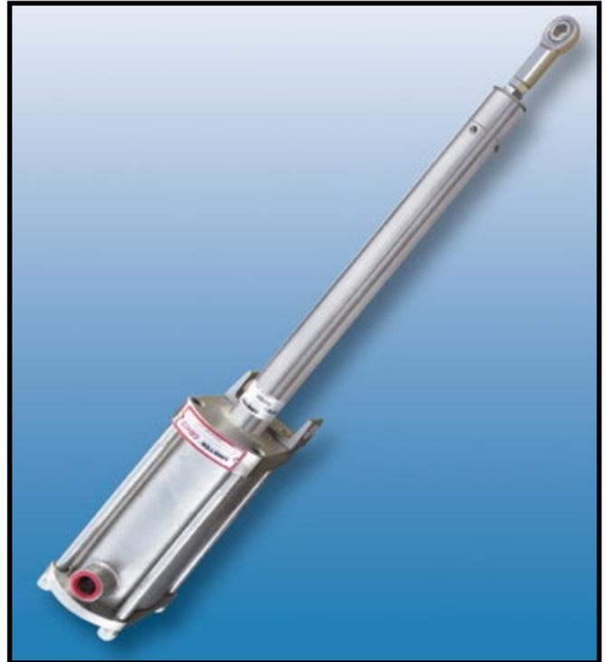
The trunnion mount bracket is positioned at the point where the head and barrel connect. A simple exchange of hardware is all that is necessary to move the trunnion mount bracket to the back cap and plug the no longer required bracket mounting holes. When ordering the 3/4" rear rod end option, the trunnion mount bracket is not supplied since it would not be required.
