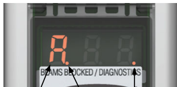
'A' in this position indicates Alignment mode Period ON indicates Blanking Configured Period ON indicates Electronic Configuration Enabled
