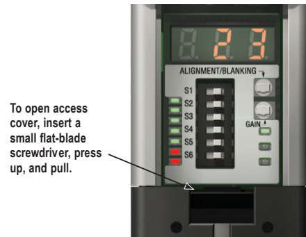
Figure 5-1. Receiver user interface. NOTE: All DIP switch positions are shown in the ON condition
