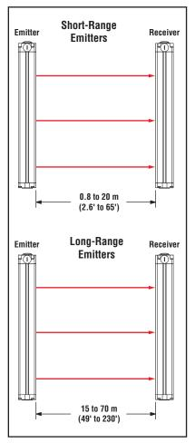
Figure 1-3. Selecting the proper emitter
