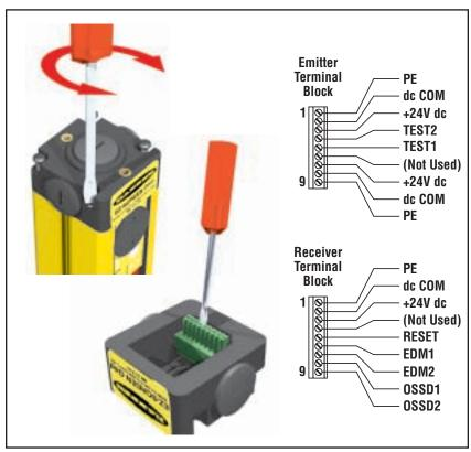
Figure 3-11. Making connections to the sensor terminal blocks
