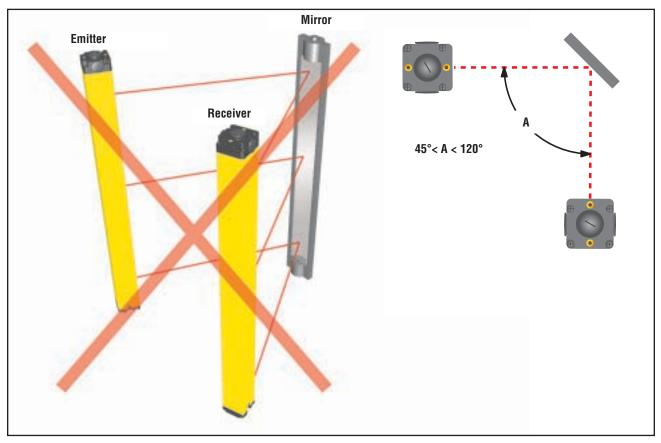
Figure 3-7. Positioning of corner mirrors
