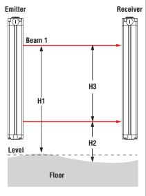
Figure 3-10. Verify required height between the top and bottom beams and the floor, throughout the length of the beam path, per applicable standards.
