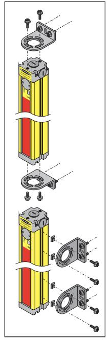
Figure 3-9. Attaching standard brackets to the end caps or side of the EZ-SCREEN
