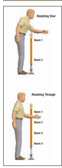
Figure 3-2. Determining D<sub>pf</sub> (reachthrough versus reach-over hazards per ANSI/RIA R15.06)
