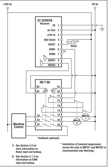
Figure 3-18. EZ-SCREEN receiver generic hookup – interface module (1-channel EDM, key reset)
