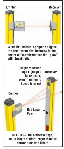
Figure 3-14. Alternate retroreflectors used for alignment
