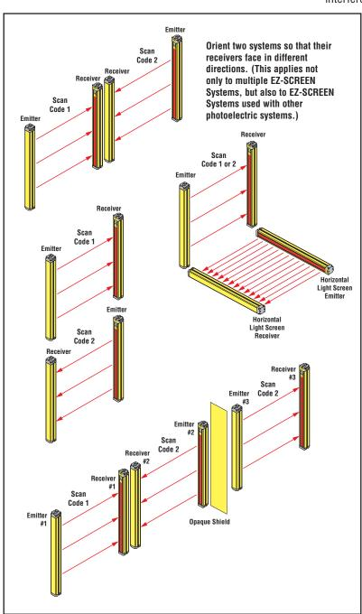
Figure 3-8. Mounting multiple EZ-SCREEN emitters and receivers to mechanically prevent optical crosstalk
