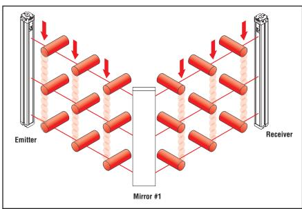
Figure 6-2. EZ-SCREEN Grid trip test with corner mirrors
