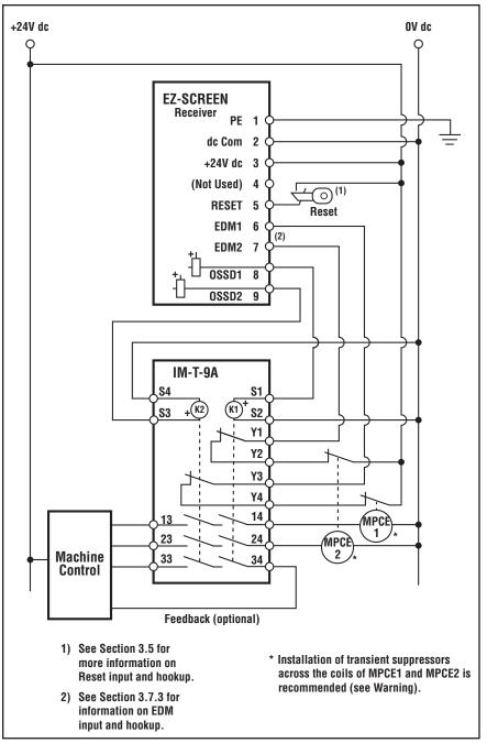
Figure 3-17. EZ-SCREEN receiver generic hookup – interface module (2-channel EDM, key reset)
