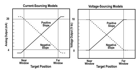
Figure 2. Positive and Negative Output Slopes
