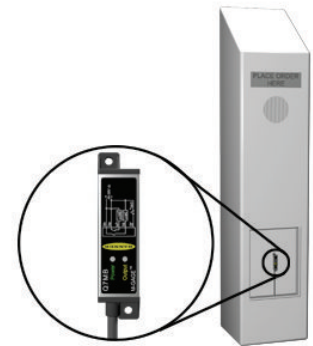
Figure 3. Installation using the mounting holes in the sensor's end caps
