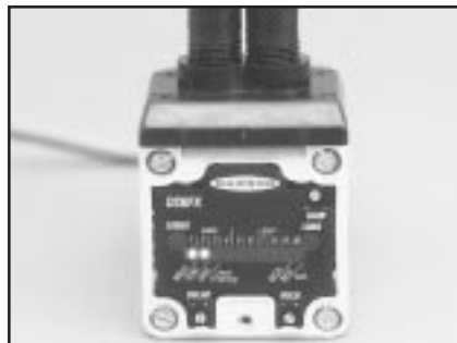
DARK condition example: D.A.T.A. system LEDs #1 and #2 lit.
