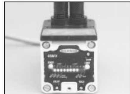
LIGHT condition example: D.A.T.A. system LEDs #1 through #8 lit.
