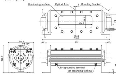
(4) Dimension of conduit entry and ON/OFF switch and end cover
