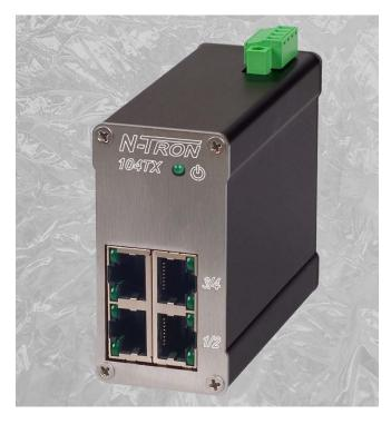
The 104TX supports up to 2,000 MAC addresses, enabling these products to support extremely sophisticated and complex network architectures.
