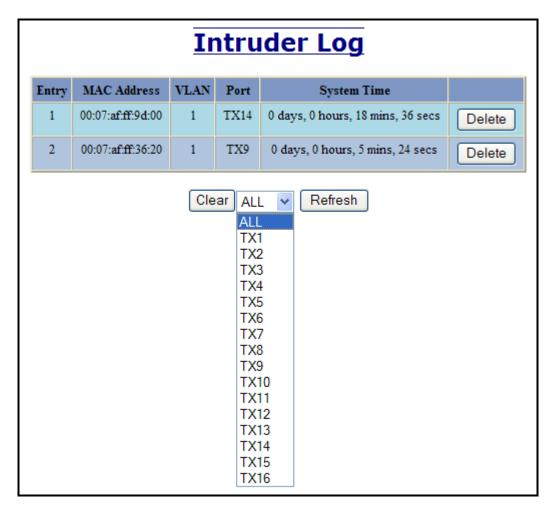
An entry can be individually removed from the log by selecting the associated Delete button. All entries or entries specific to a port can also be removed from the log by choosing the option in the dropdown list and then selecting the Clear button.
