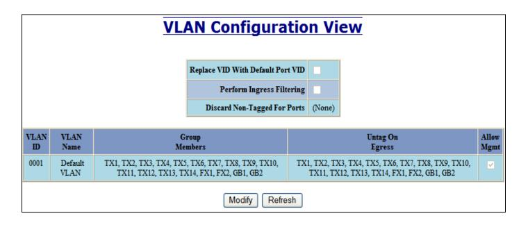
Clicking on the "Modify" button allows one to add a new VLAN:
