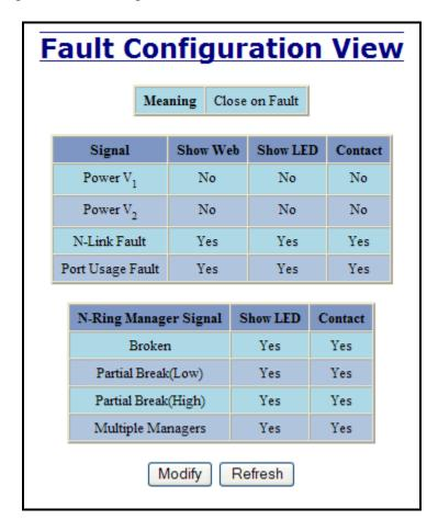
Note: V<sub>1</sub> and V<sub>2</sub> Power Faults are disabled in factory defaults.
