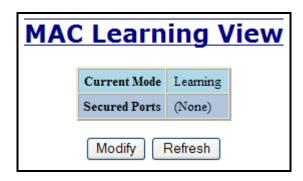
In 'Locked' mode, 'Secured Ports' shows the ports that are presently secured. *Note: when N-Ring and/or N-Link are used, the N-Ring/N-Link ports will not have MAC Security enabled.*
