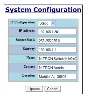
If the IP Configuration mode is set to DHCP and the Fallback IP address is changed from the default IP address, then the switch will use the Fallback addresses if the IP configuration isn't received from a DHCP server in 2 minutes after initial boot. If Fallback address is used, DHCP Client will stop sending requests. If the IP Configuration is received from a DHCP server, it will never fallback, even if the lease is lost.
