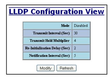
Note: A redundant network topology will have one or more blocking ports to prevent looping and broadcast storms. LLDP will not receive neighbor information into a blocked port, though the LLDP information will be transmitted out of a blocked port. Therefore, the switch that has the blocked port will not know about the neighbor on the other side of the blocked port, but the neighbor will know about the switch that has the blocked port.
