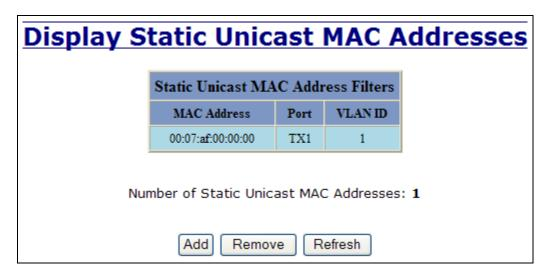
Following the Remove button on the example above, an administrator can select a static MAC address from the list using a pull-down menu. After selecting the MAC address, the administrator needs to press the Remove button on the page to remove the entry
