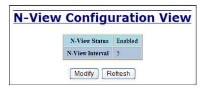
Following the Modify button on the above example, the administrator can modify the variable to change the frequency with which N-View reports information. Increasing the interval will slow the update rate. Decreasing the interval will allow N-View to report more frequently. Additionally, you may Disable or Enable N-View altogether.
