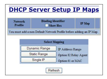
The Dynamic Range type of mapping is used to create a range of dynamic IP addresses for requesting clients. The following information is required:
