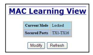
The Modify button allows the administrator to change the current mode. When transitioning from 'Learning' to 'Locked', the Address Resolution Logic (ARL) table represents the authorized MAC addresses, with the addition of any manually entered addresses (refer to Authorization List section below). Transitioning from 'Locked' to 'Learning', clears the ARL for all ports.
