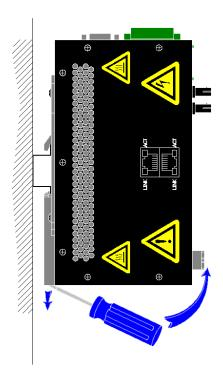
To mount the unit to the 35mm din-rail, place top edge of the bracket on the back of the unit against the din-rail at an upward angle. Lower the bottom of the unit until it snaps into place.
