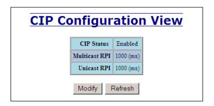
Following the Modify button on the above example, the administrator can modify the variables. Additionally, you may Disable or Enable CIP altogether.
