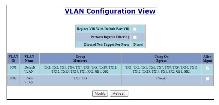
The ports of "New VLAN" may be added back to "Default VLAN" to create overlapping VLANs.
