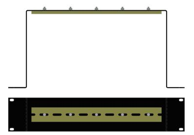
Most N-Tron™ products are designed to be mounted on industry standard 35mm DIN-Rail. However, DIN-Rail mounting may not be suitable for all applications. Our Universal Rack Mount Kit (P/N: URMK) may be used to mount the 7018 Series to standard 19" racks as an option.
