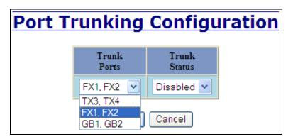
**Note:** RSTP must be disabled in order to use the Trunking feature. Two ports of the same speed can constitute a valid trunk. Only 1 Trunk per switch can be created.
