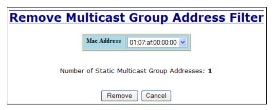
**Note:** If there are multiple ports on different VLANs, the 7018 will apply the static multicast address to the lowest VLAN-ID that is associated with one of the ports assigned to the static multicast address. So if the lowest VLAN-ID contains all the ports assigned to the static multicast address (an umbrella VLAN), it will function for all those ports with no problems. This can be achieved with overlapping VLANs.
