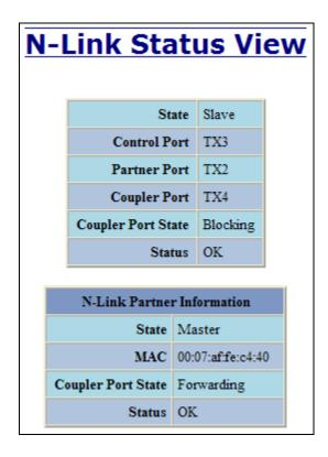
Below is an example of N-Link Status from an N-Link Master and Slave where the Primary Coupler link is broken:
