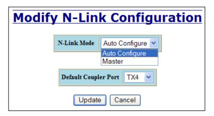
If N-Link mode is "Master", then the administrator must configure the Control Port (default: TX3) and the Primary Coupler Port (default: TX4).
