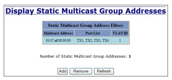
Following the Remove button on the example above, the administrator will be presented with a list of Multicast Group Addresses that are configured on the switch. Using the pull-down menu, the administrator should select the desired address to be removed. Then click on the Remove button at the bottom of the page.
