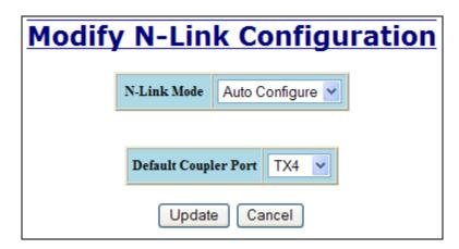
The port configured as the Default Coupler Port will be used as the Standby Coupler port if the switch detects an N-Link Master and becomes an N-Link Slave.
