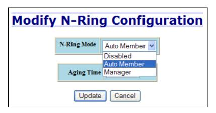
If N-Ring Mode is "Manager", then a pull-down allows selection of available ports TX1/TX2, TX15/TX16 (FX1/FX2 on 7018FX2), or GB1/GB2 as N-Ring ports.
