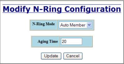
The N-Ring Aging Time has a default of 20 seconds and is separate from the Bridging Aging Time. N-Ring Aging Time is used when the switch is an N-Ring Manager or becomes an active N-Ring Member, and in either case N-Ring status includes for example:
