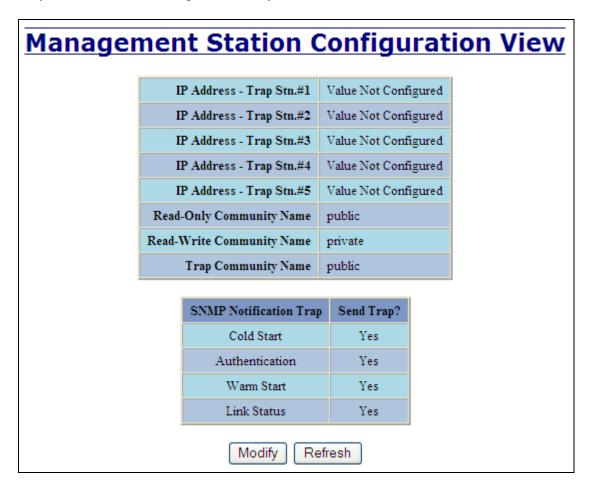
By selecting the Modify button, you will be able to change any of the fields listed. This allows the user to set an IP address for a Trap station or change the Community Names. If the SNMP Notification Trap is enabled, systems that are listed as a Trap station will be sent the corresponding notification trap. To restore a Trap to "Value Not Configured", enter '0.0.0.0'.
