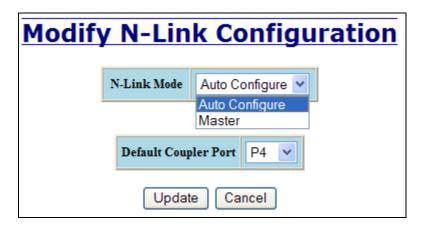
If N-Link mode is "Master", then the administrator must configure the Control Port (default: P3) and the Primary Coupler Port (default: P4).
