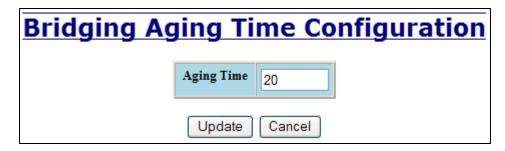
**Note:** If the switch is an active participant of an N-Ring, then the N-Ring Aging Time will be used instead of the Bridging Aging Time.
