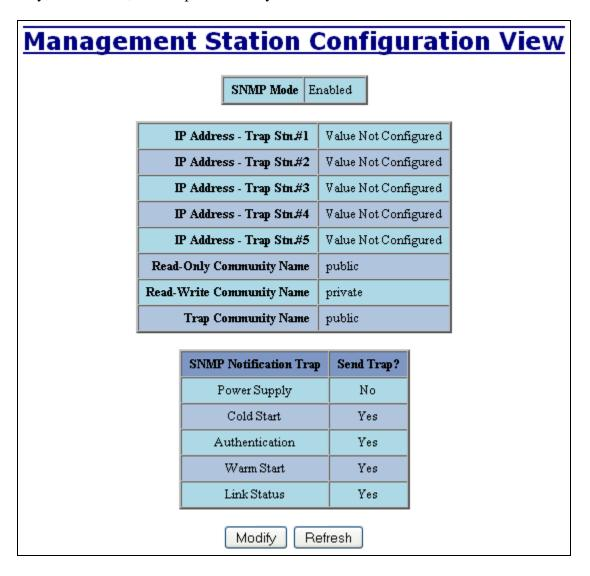
By selecting the Modify button, you will be able to change any of the fields listed. This allows the user to set an IP address for a Trap station or change the Community Names. If the SNMP Notification Trap is enabled, systems that are listed as a Trap station will be sent the corresponding notification trap. To restore a Trap to "Value Not Configured", enter '0.0.0.0'.
