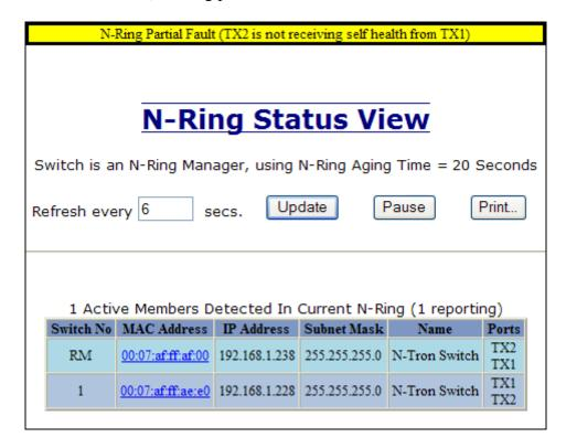
The screenshot below shows N-Ring Manager Status when a 'Lower' N-Ring Port (TX1, TX7/FX1, or GB1) is not receiving self health frames all the way around the N-Ring, though the other (high TX2, TX8/FX2, or GB2) N-Ring port is:
