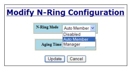
If N-Ring Mode is "Manager", then a pull-down allows selection of available ports P1/P2, P23/P24, and P25/P26 as N-Ring ports.
