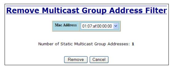
**Note:** If there are multiple ports on different VLANs, the 7026 will apply the static multicast address to the lowest VLAN-ID that is associated with one of the ports assigned to the static multicast address. So if the lowest VLAN-ID contains all the ports assigned to the static multicast address (an umbrella VLAN), it will function for all those ports with no problems. This can be achieved with overlapping VLANs.
