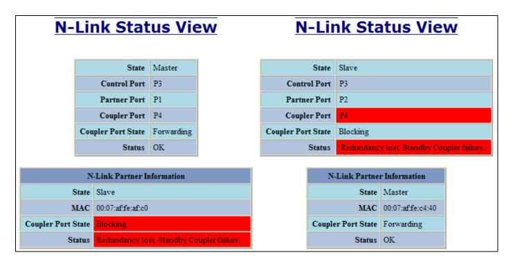
Below is an example of N-Link Status from an N-Link Master and Slave where the Control link is broken:
