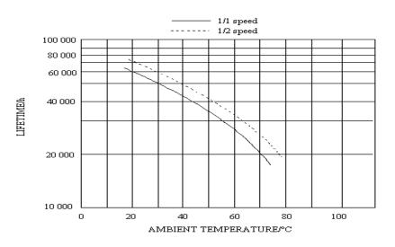
Typical lifetime of the cooling fan versus ambient temperature
