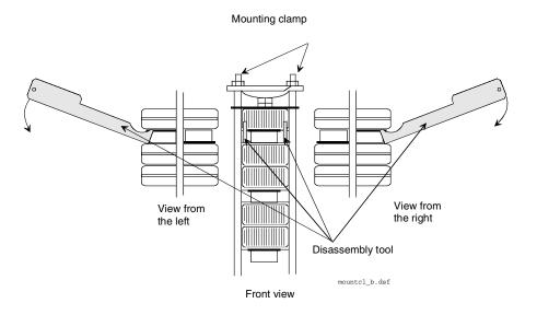
How to use the disassembly tool
