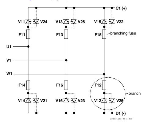
Anti-parallel B6-bridges with branching fuses
