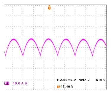
Six current pulses in positive direction
