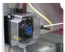
Cooling air pressure switch
