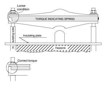
Aluminum spring with welded indicating spring
