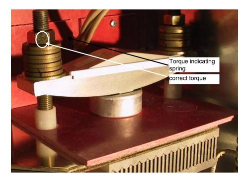
Mounting clamp, correct torque
