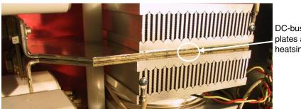
DC-busbar plates and heatsinks
