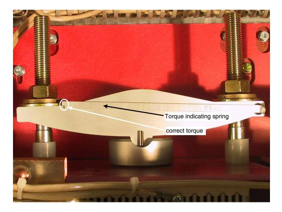
Mounting clamp; correct torque
