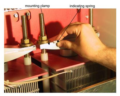
Handling of indicating spring and mounting clamp
