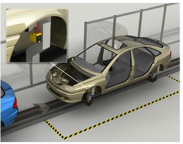
Using the tower light notification system reduces the need for technicians or managers to constantly check each production line.
