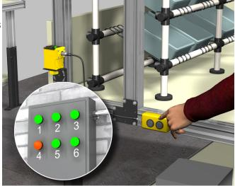
As the needs of the production operators changed, the wireless call-for-parts system is easy to move and reinstall.
