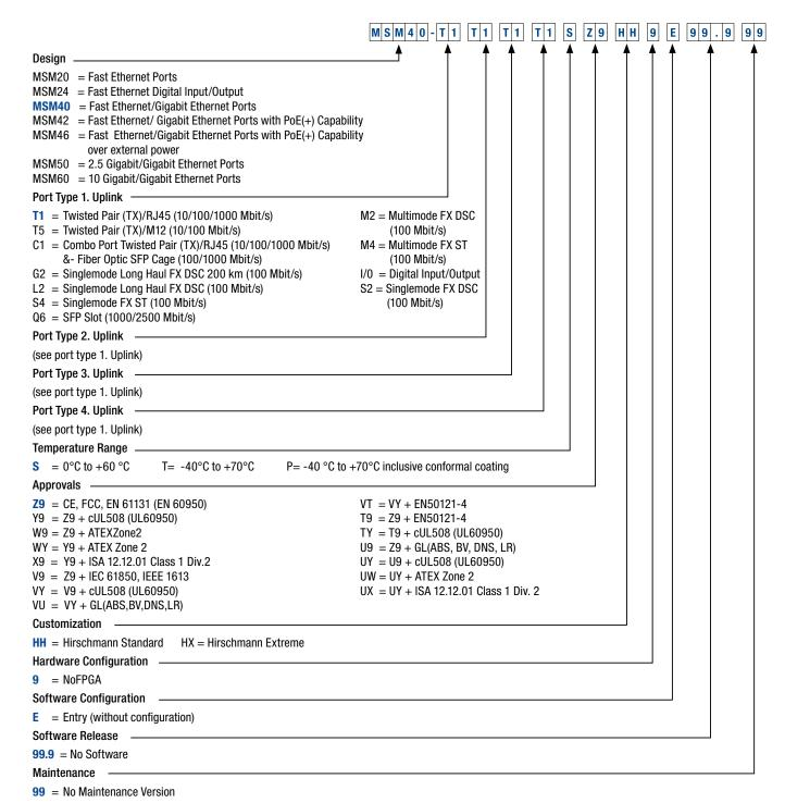
NOTE: The categories (Customization, Hardware Configuration, Software Configuration and Software Release) are optional.
