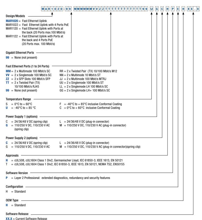
NOTE: The last three part number categories (Configuration, 0EM Type and Software Release) are optional.
