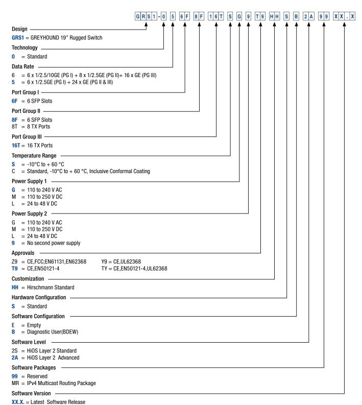
NOTE: The last four categories (OEM type, configurations, software version and software release) are optional.
