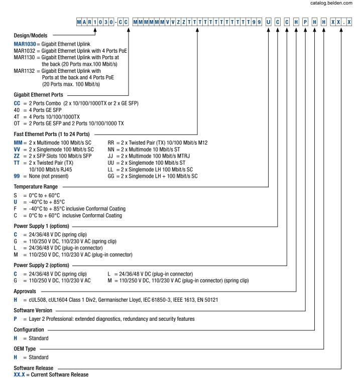
NOTE: The last three part number categories (Configuration, 0EM Type and Software Release) are optional
