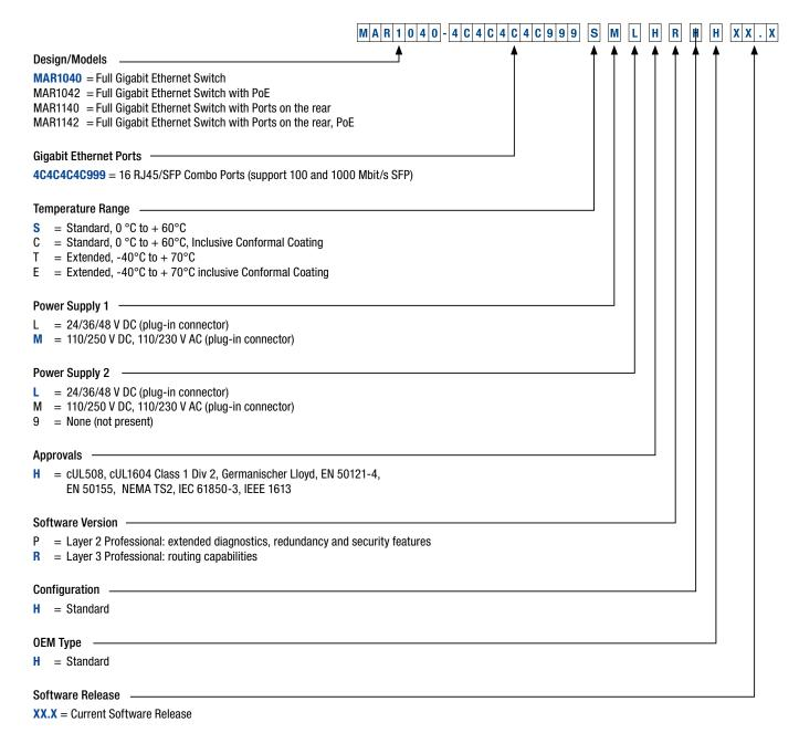
NOTE: The last three part number categories (Configuration, OEM Type and Software Release) are optional.
