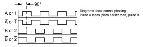
Connect the encoder output channel that leads when the drive runs Forward to BTAC terminal A. Connect the output channel that trails to BTAC terminal B.
