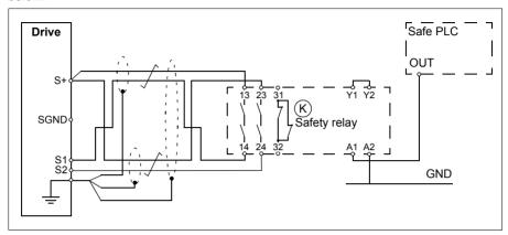
An example of a Safe torque off wiring with external +24 V DC power supply is shown below.
