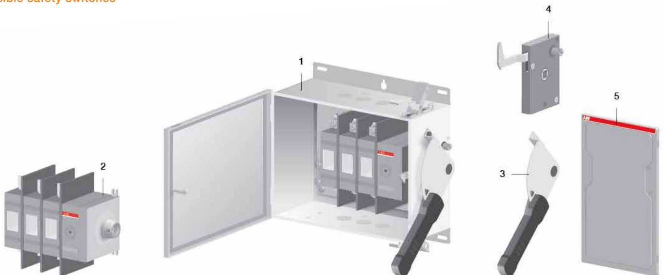
1 Non-fusible safety switch | 2 Switch-disconnect | 3 Handle kit | 4 Door interlock mechanism | 5 Door assembly
