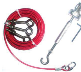
Tensioner / Gripper Assembly Allen Key 4mm Quick Link (QL) For up to 50m. spans ,one rope end is terminated with a thimble and permanent clamp. For over 50m. spans, 2 Tensioner / Gripper assemblies are supplied (no Quick Link).
