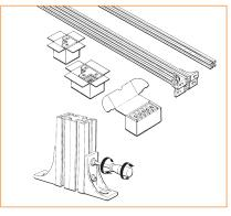
tion and mechanically lock the fixture into the profile. Make sure that the nut has turned correctly.
