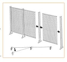
Lock the top of the mesh using NL3 net-locks; this way the mesh is secured, stabilized and electrically grounded.
