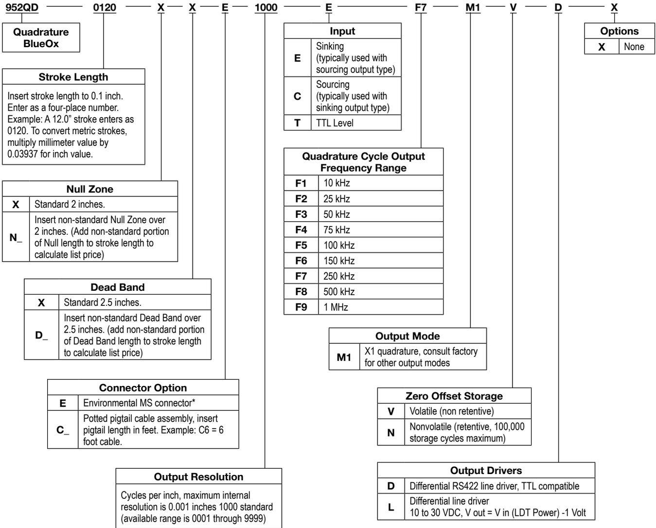
\* If option E (environmental connector) is selected, mating connector and/or cable assembly must be ordered separately.
