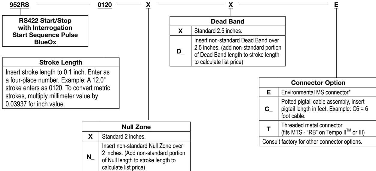
\* If option E (environmental connector) is selected, mating connector and/or cable assembly must be ordered separately.
