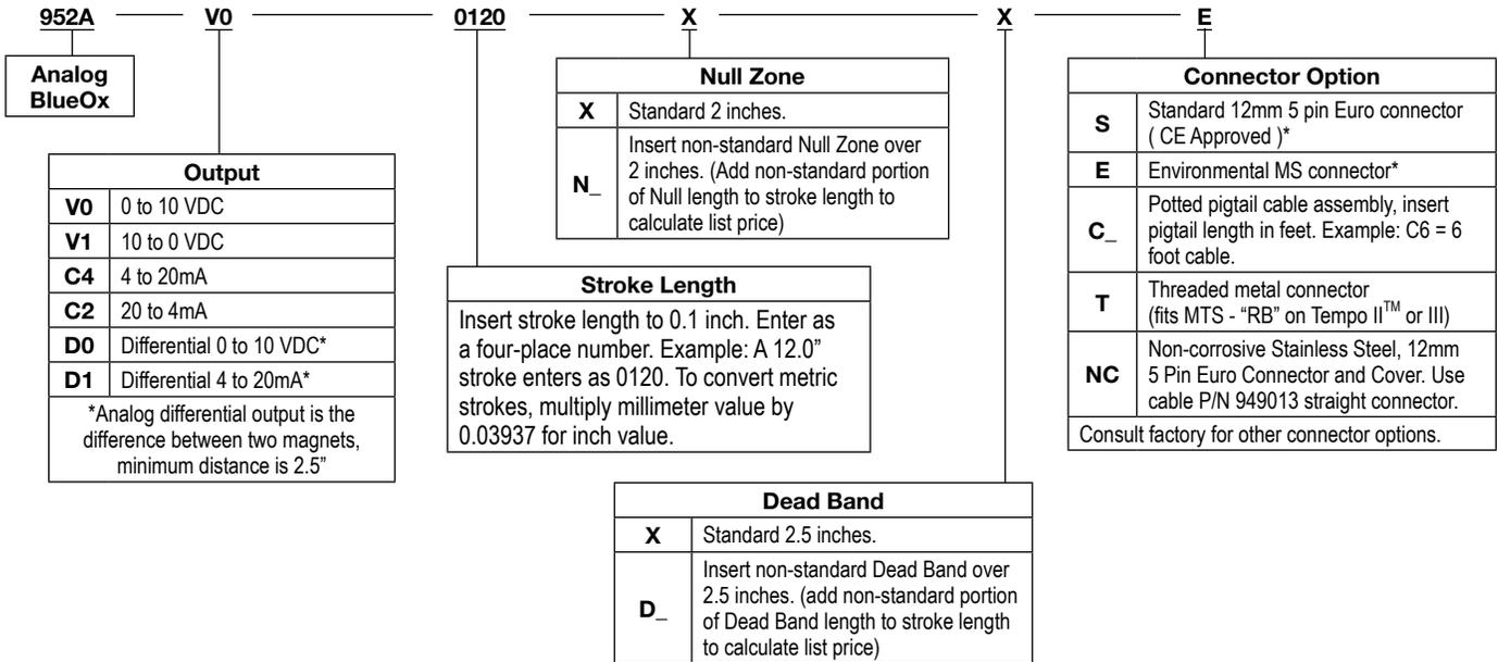
**Note 1:** On unsupported stroke lengths greater than 4 feet, rod support bracket(s) and a special magnet should be used.
