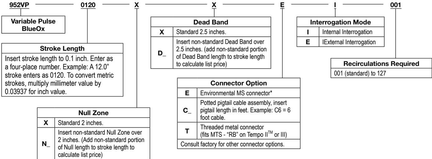
\* If option E (environmental connector) is selected, mating connector and/or cable assembly must be ordered separately.
