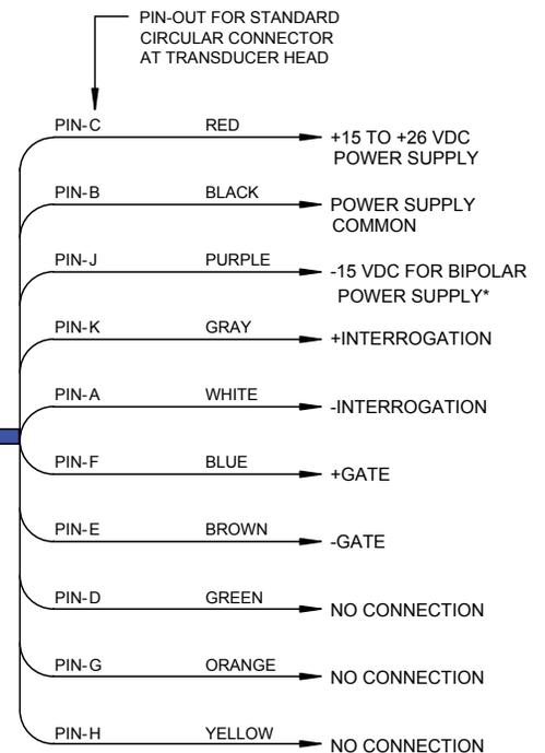
\* FOR UNIPOLAR POWER SUPPLY, IT IS RECOMMENDED TO CONNECT THIS WIRE TO POWER SUPPLY COMMON
