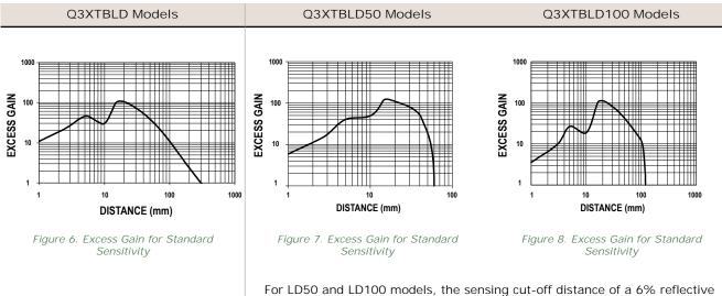
For LD50 and LD100 models, the sensing cut-off distance of a 6% reflective black card will be 95% of the sensing cut-off distance of a 90% reflective white card.
