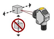
Figure 4. Optimal Orientation of Target to Sensor
