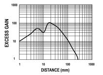
Figure 10. Excess Gain for Standard Sensitivity
