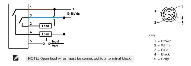
NOTE: The input wire function is user-selectable; see the Instruction Manual for details. The default for the input wire function is off (disabled).
