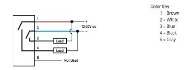
Note: Cabled wiring diagrams are shown. Quick disconnect (QD) wiring diagrams are functionally identical.
