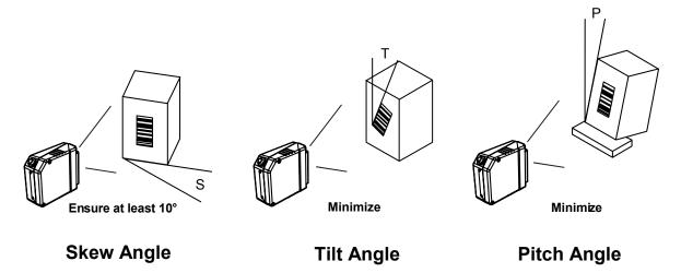
Figure 4. Skew, Tilt, and Pitch Angles
