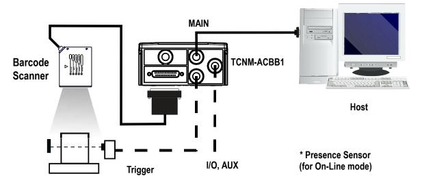
Figure 1. Barcode scanner in a standalone layout
