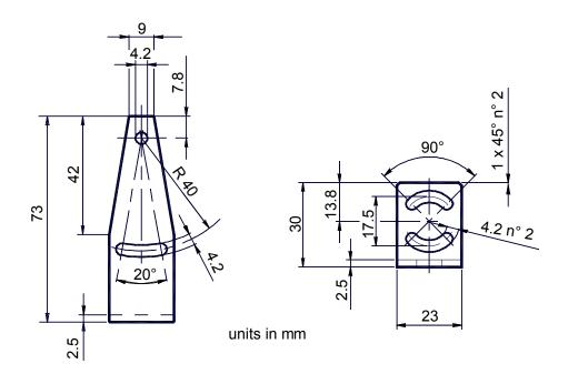
Figure 6. Mounting Bracket Overall Dimensions
