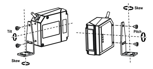
Figure 3. Positioning with mounting bracket
