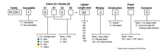
Density (D) is defined by the quantity of LEDs populated on the circuit. For example, at 100% density, there are 18 LEDs per 285 mm, and at 50% density, there are 9 LEDs per 285 mm. The lumen output decreases proportionally with density.
