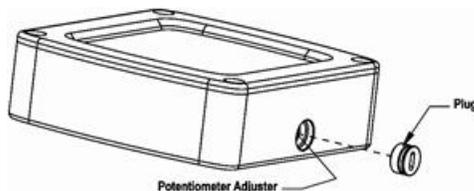
Figure 1. Potentiometer adjuster
