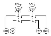
Figure 2. Series connection of multiple E-stop switches
