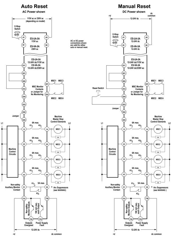
Figure 5. Wiring for 1-Channel E-Stop Applications
