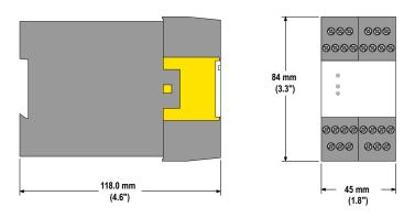
Figure 6. Dimensions in Millimeters (Inches)
