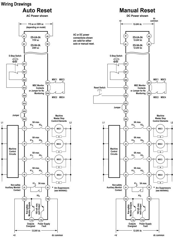
Figure 4. Wiring for 2-Channel E-Stop Applications
