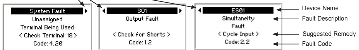
Figure 55. Current Fault screens—OBI
