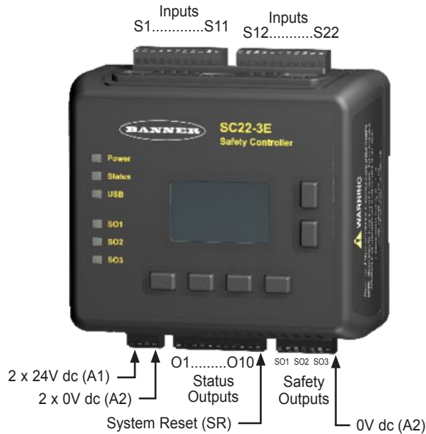
Figure 10. Input and output terminal locations
