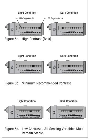
Figure 5. Sensitivity Adjustment; Light and Dark Condition Settings Should be Equally Spaced from the Switch Point The 10-element moving LED light bar displays received light signal strength, relative to the switch point setting. This display makes sensitivity adjustment extremely easy and accurate.
