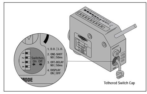
The four switches located behind the tethered cap labeled "MODE" are used to select the functions shown in the table below.
