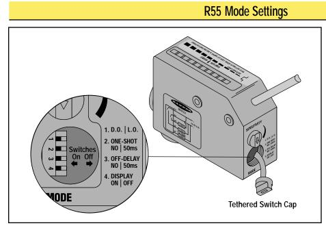
The four switches located behind the tethered cap labeled "MODE" are used to select the functions shown in the table below.
