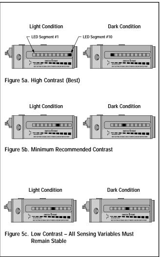
Figure 5. Sensitivity Adjustment; Light and Dark Condition Settings Should be Equally Spaced from the Switch Point The 10-element moving LED light bar displays received light signal
