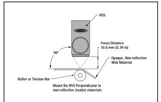
Figure 4a. Mounting for sensing opaque non-reflective materials
