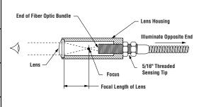
Lenses are most efficient when they are located slightly beyond their focal length distance from the sensing end of the fiber optic bundle. The easiest way to focus a lens is to treat it like a magnifying glass.
