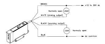
NOTE: These sensors will operate normally if the supply voltage polarity is reversed; however, the white and black wires must always be wired as shown above.
