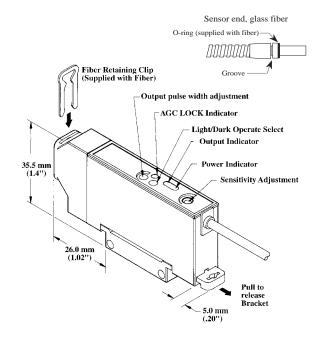
**Operating temperature range:** -40° to +70°C (-40° to +158°F). **Maximum relative humidity** 90% at 50°C (non-condensing).
