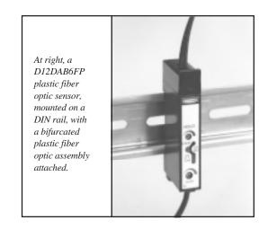
A switch on the sensor's top panel selects either light- or dark-operate. When light-operate is selected, output occurs on a dark-to-light transition. When dark-operate is selected, output occurs on a light-to-dark transition.
