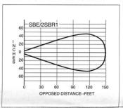
Model **2SBR1** receiver is used with the **SBE** emitter, the same emitter used with the 1 millisecond 3- & 4-wire receiver model **SBR1**. The response time, however, is determined by the receiver, and is 10 milliseconds. This pair will
