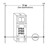
MULTI-BEAM 2-wire sensors wire in series with an appropriate load. This combination, in turn, wires directly across the ac line. A 2-wire sensor may be connected exactly like a mechanical limit switch.
