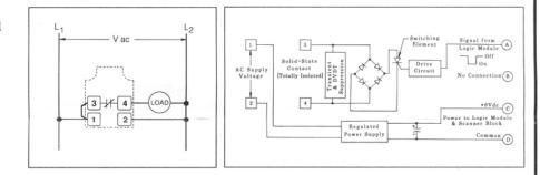
Model PBAQ is identical to model PBA (page 1) except that the solid-state output contact is normally closed instead of normally open. It is used where it is necessary to have the load deenergize when something is sensed (e.g.- one shot pulse to de-energize load). When no timing logic is involved, model LM3 can program any power block for normally open or normally closed operation via the light/dark operate jumper.
