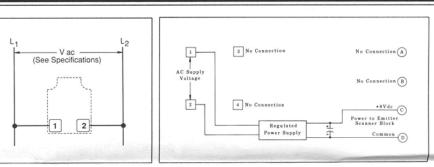
These power blocks are used to power emitter-only scanner blocks. Models PBA-1, PBB-1, and PBD-1 save the cost of the output circuitry that must be included in other power block models. (These other power blocks may, however, be used to power emitter-only scanner blocks, with the output switching circuitry going unused.)
