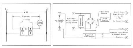
Power block models PBAT and PBBT have an isolated solid-state output switch which may be used to switch either ac or dc. The switch is rated at 100mA maximum, and there is no capacity for inrush. As a result, these power blocks usually should not be used to switch ac inductive loads. However, 100mA is enough capacity to switch many inductive *dc* loads like small relays and solenoids.
