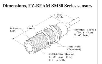
Quick Disconnect fitting adds .35" (9 mm) in overall length to QD models. QD models require Quick Disconnect cable (order separately; see Specifications section for information).
