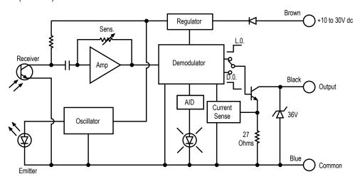
SMI912 Series sensors feature rugged, encapsulated construction, along with adjustable sensitivity and switchable light or dark operate. They also include Banner's exclusive Alignment Indicating Device system, which lights an indicator LED whenever the sensor "sees" its modulated light source, and pulses at a rate proportional to the received light signal strength.
