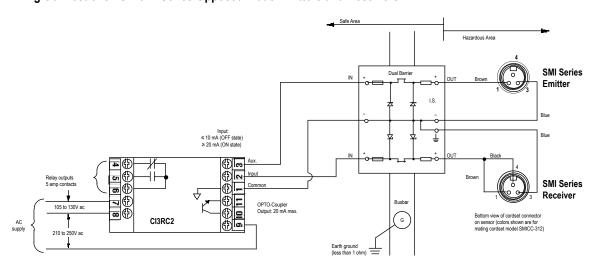
Wiring Connections - All Other SMI912 Series Sensors
