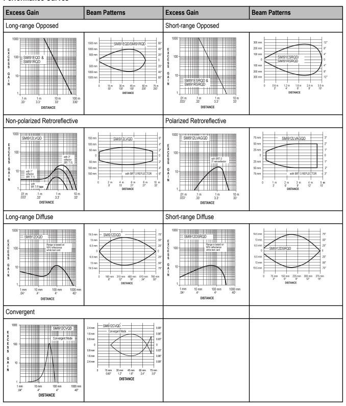
Retroreflective performance based on use of a model BRT-3 retroreflector (3" diameter). Actual sensing range may be more or less than specified, depending on the efficiency and reflective area of the retroreflector used.
