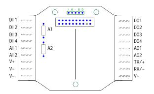
RX/-. Serial comms line for Gateways and DX85s only. No connection for Nodes.
