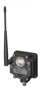
SureCross® MultiHop data radios are wireless industrial communication devices used to extend the range of a Modbus or other serial communication network.
