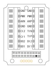
AXN, AXP. Not used. Do not make any wiring connections to these terminals.
