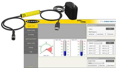
The User Configuration Tool (UCT) offers an easy way to link I/O points in your wireless network, view I/O register values graphically, and set system communication parameters when a host system is not part of the wireless network. Download the most recent revisions of the UCT software from Banner Engineering's website: <http://www.bannerengineering.com/wireless>.
