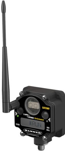
The SureCross® wireless system is a radio frequency network with integrated I/O that can operate in most environments and eliminate the need for wiring runs. Wireless networks are formed around a Gateway, which acts as the wireless network master device, and one or more Nodes.
