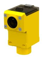
The convergent sensor is ideal for reflective sensing of very small parts or profiles, and can accurately sense the position of parts approaching from the side. The sensor will ignore all but the most highly reflective objects that are outside the sensing range.
