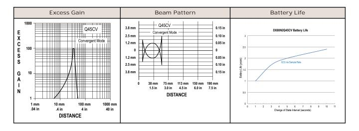
Performance curves are based on a 90% reflectance white test card.
