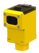
The visible red sensing beam of the retroreflective sensor makes it very easy to align. The sensor polarizes the emitted light and filters out unwanted reflections, making sensing possible in applications otherwise considered unsuited to retroreflective sensing. Performance is specified using the model BRT-3 3-inch reflector (see the Accessories section of your current Banner catalog for further information).
