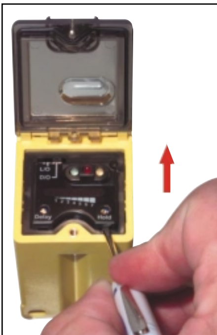
Figure 2. Insert a small screwdriver into the slot and lift the black cover to remove.
