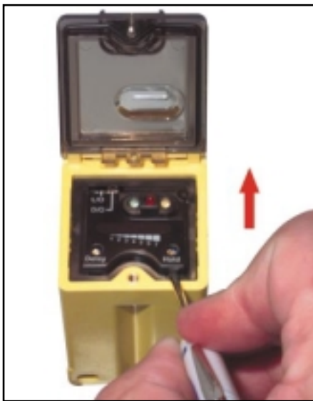
Figure 5. Insert a small screwdriver into the slot and lift the black cover to remove.
