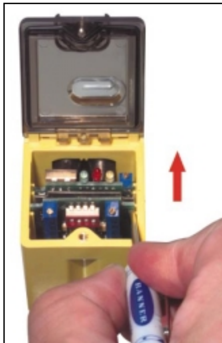
Figure 3. Using the small screwdriver in the module slot if necessary to nudge the module loose, lift the module up and out.
