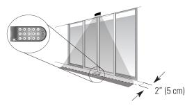
Use the 2" width mark on the RC Duo 2 to determine e.g. when the infrared safety curtain is 2" from the face of a sliding door.
