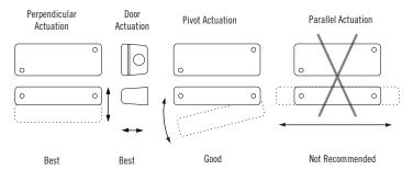
Three configurations are appropriate for interlock applications. The parallel actuation can result in on/off/on signal if the actuator passes by the switch rather than coming to rest in proximity to it. This is NOT a recommended configuration for interlock applications.
