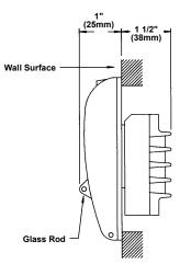
NOTE: Flush mtg. unit fits 4" square box and plaster cover with single gang opening having overall min. depth of 2 1/4"
