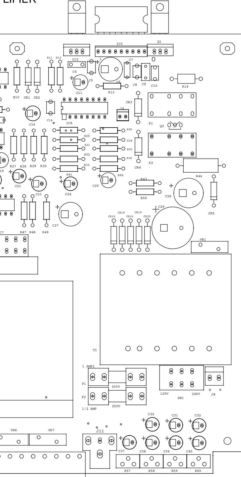
Figure 5-1. Model 300VSC Mother Board Parts Location.
