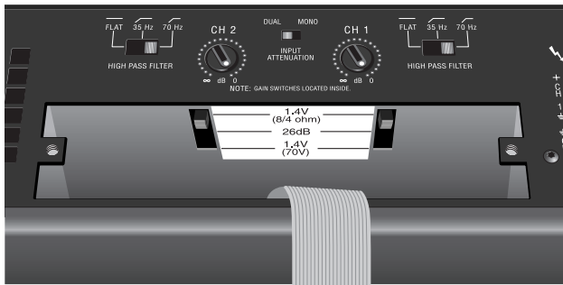
Figure 5.1 Input Sensitivity Switches for CTS 600/1200
