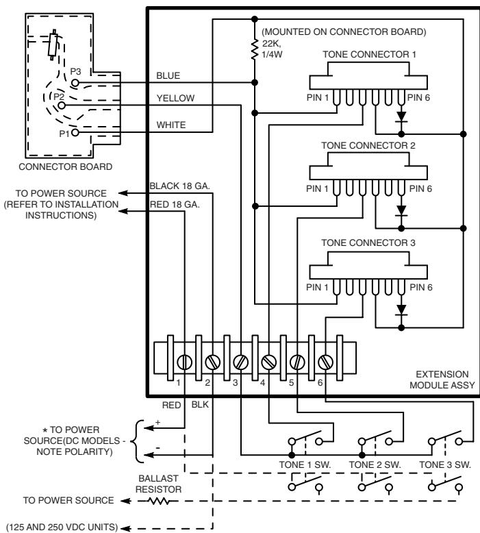
\* DASHED LINES INDICATE CONNECTIONS FOR 125 AND 250 VDC UNITS.
