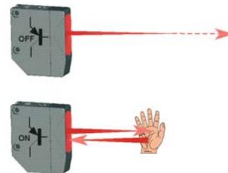
A proximity sensor normally operates in light mode: the output is activated when an object enters the detection area and reflects light emitted by the sensor.
