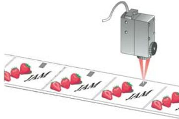
Contrast sensors are mainly used in automatic packaging machines for registration mark detection to synchronize folding, cutting and welding.
