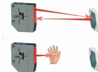
When installing sensors which detect reflected light, make sure that unwanted light reflections from nearby surfaces, such as the floor, walls, reflective machinery or stainless steel, do not reach the optical receiver.
