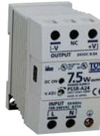
When using a switching power supply, be sure to ground the FG terminal to eliminate high-frequency noise. The power supply should include an insulating transformer, not an autotransformer.
