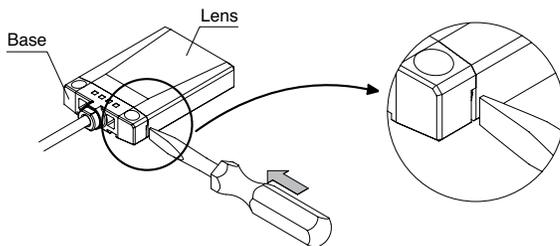
2. Twist the screwdriver and disengage the lens from the base.
