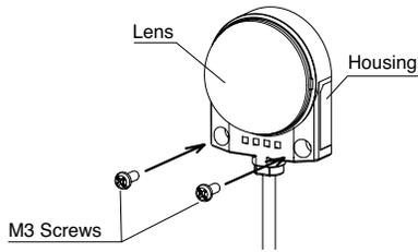
Note: The standard dome lens is not removable. Do not attempt to remove or damage may occur. However, the jumbo dome lens is removable and replaceable.
