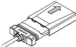
4. Insert the edge of a marking film into the gap between the base and the diffusion plate, and place the marking film on top of the diffusion plate.
