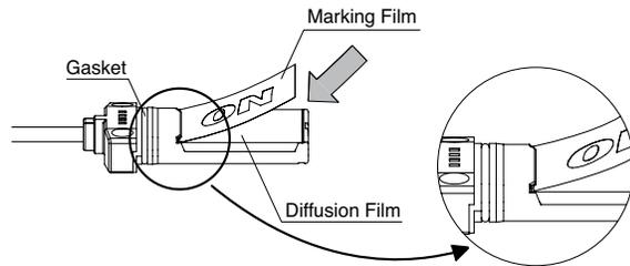
5. Replace the lens. Ensure that the lens is installed snugly.
