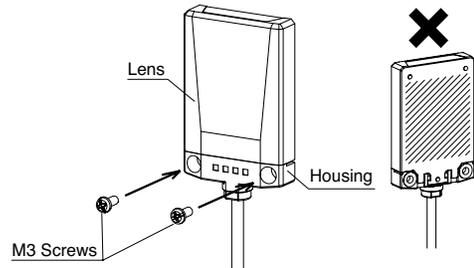
Note 1: Do not install the LH indicator by attaching the lens only, such as by taping down on the lens as the internal components may come loose.
