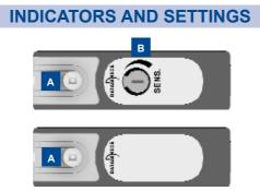
Single-turn trimmer for sensitivity adjustment. Rotate clockwise to increase the operating distance.
